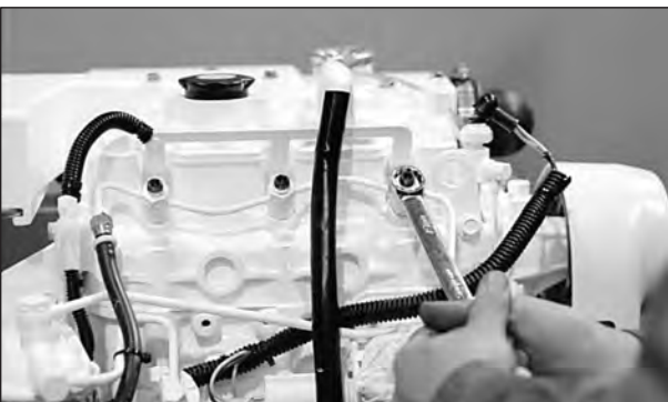
Figure 14: Remove return line nuts.
