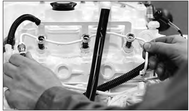
Figure 15: Remove return line.
