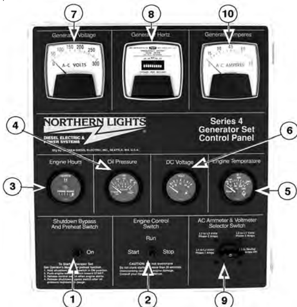
Figure 3-C: Series 4 Generator Control Panel
