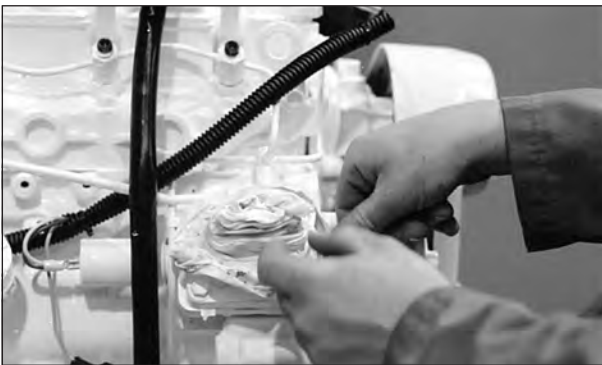
Figure 13: Cover lines, inlets and injection pump outlets.
