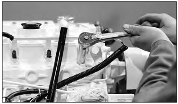
Figure 18: Reinstall injector. Torque to proper tightness.
