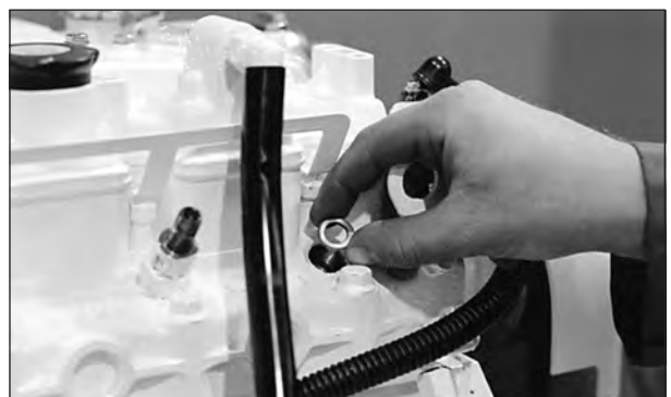
Figure 17: Remove and replace copper sealing washer.
