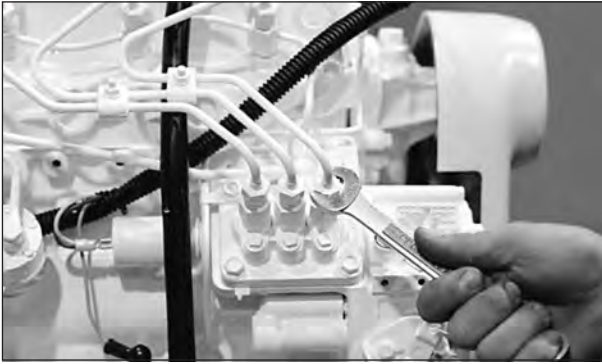
Figure 11: Remove delivery line flare nuts.
