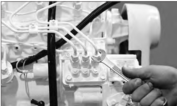
Figure 10: Remove delivery line flare nuts.
