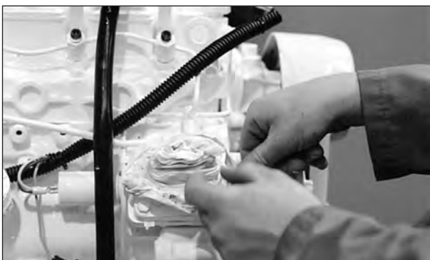
Figure 12: Cover lines, inlets and injection pump outlets.
