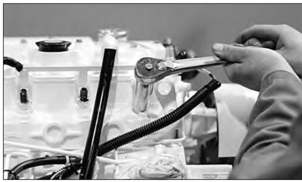
Figure 17: Reinstall injector. Torque to proper tightness.
