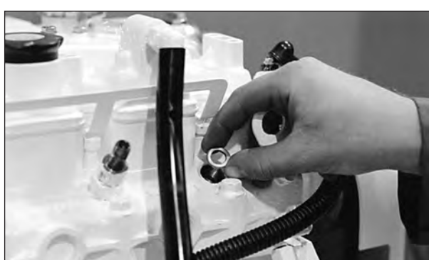
Figure 16: Remove and replace copper sealing washer.
