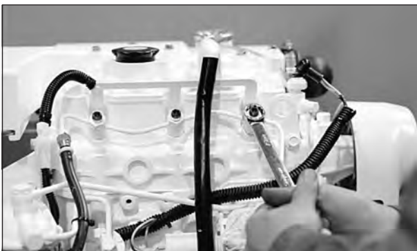
Figure 13: Remove return line nuts.
