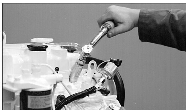
Figure 20: Reinstall injector. Torque to proper tightness.
