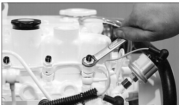
Figure 16: Remove return line nuts.
