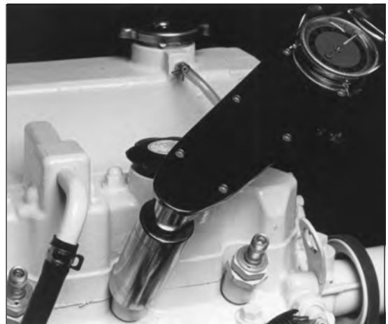
Figure 18: Reinstall injector. Torque to proper tightness.
