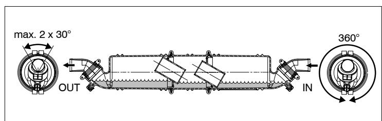
For a proper working it is essential that the OUT part of the housing and both the inner parts are placed in the positions as shown in the illustration. A deviation of maximum 30° to either side is permitted.
