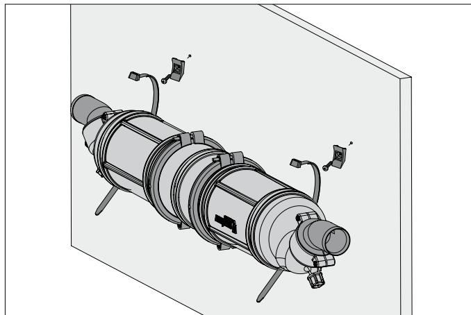
The waterlock has slots in which the ty-raps® should be fitted.
