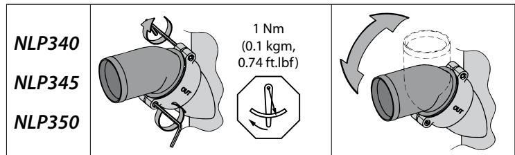
**Loosen the bolts before turning the hose connections!** Tighten the hose connections to a torque of 1 Nm (0.74 ft-lb, 142 oz-in).
