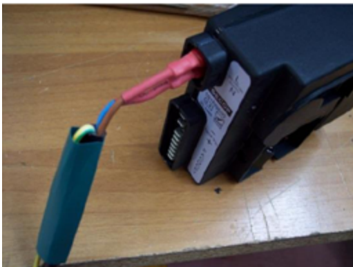
Figure 11: Detail of double insulated connection
