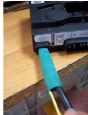
Figure 11: Detail of double insulated connection
