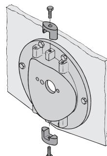
Install de thrust tunnel onto the flange with the supplied bolts en washers.
