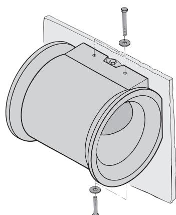
**IMPORTANT:** The centerline of the drill pattern must be **precisely** horizontally and at least 150mm below the waterline.
