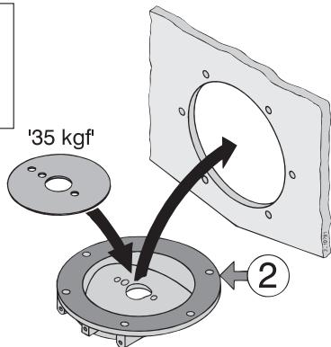
Install the flange with the supplied bolts, nuts and washers.
