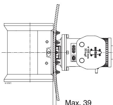
In case that the available height at the stern is insufficient for the installation of the stern thruster a sloped surface can be made to install the stern thruster. Than keep in mind that the thrust tunnel must be protected against the forces caused by the water flow during normal cruising.
