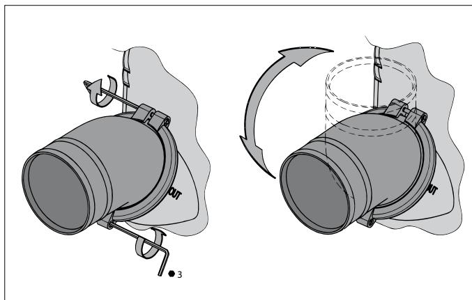
In order to achieve the ideal connection between the hoses and the waterlock, both hose connections turn through 360 degrees.
