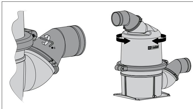
The top portion of the waterlock can be turned in a 360° radius.
