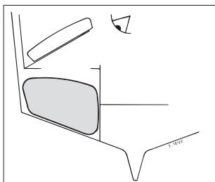
The tank should always be installed above the maximum bilge water level.
