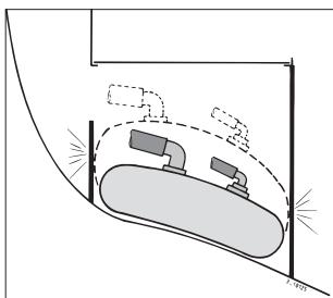
The hull and sides must be smooth. If not, then cover them with felt or foam.
